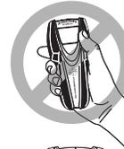
Keep tool flat against the wall and do not rock or tilt the tool when scanning.
